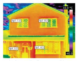
**BEFORE** and **AFTER**: The above thermal images clearly demonstrate the advantages of installing new energy efficient windows. The heat loss temperature of the living room window is  $1.3^{\circ}$ C before and  $-4.5^{\circ}$ C after the new windows were fitted - a significant reduction.
